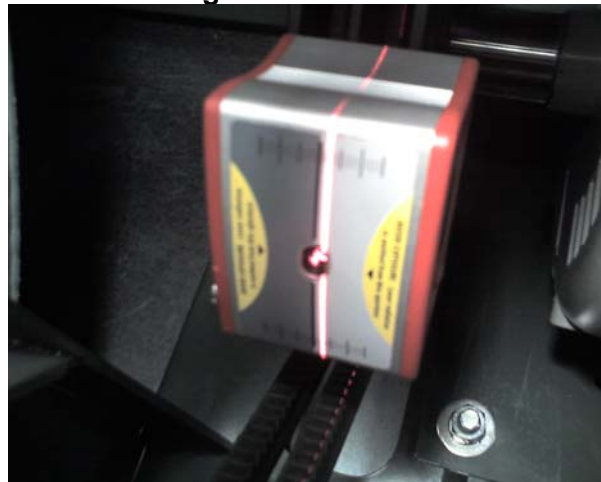
Motor Sheave Alignment in area with 5 mil runout
