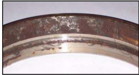
This is the condition of the spindle bearings after removing them. The coolant line had ruptured and purged all of the bearing grease out of the bearings. The coolant also continued running and caused the contamination and rust to develop.
